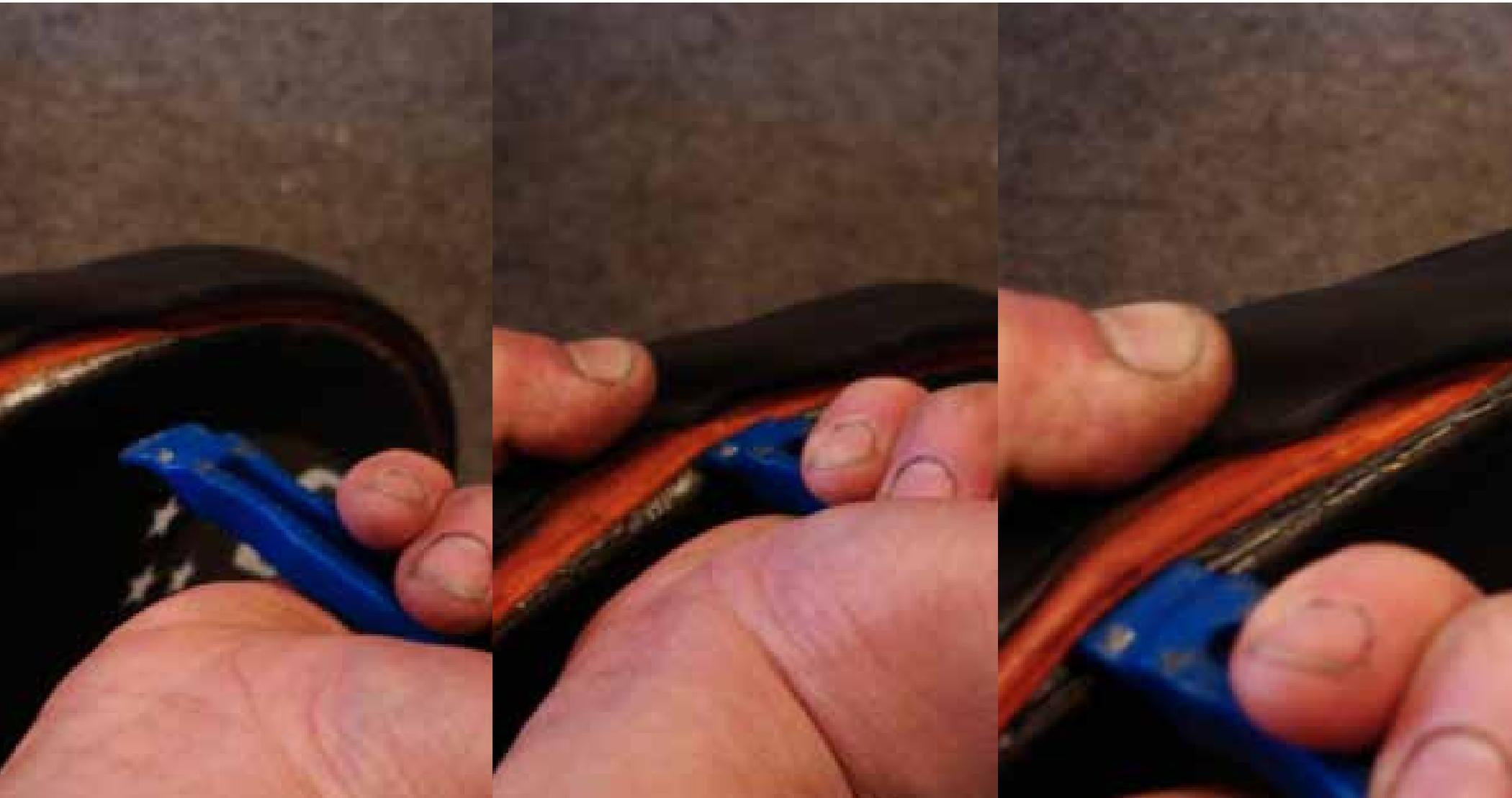
First, once you get a flat, downshift the bike to your hardest gear to allow the wheel to come out of the dropout easier (and also easier when putting it back in later). Then, after getting the wheel out take tire lever with somewhat of an edge on it and pull the tire back and run the tire lever back and forth to break up the glue "threads" showing to get the lever between the tire and the rim itself.
