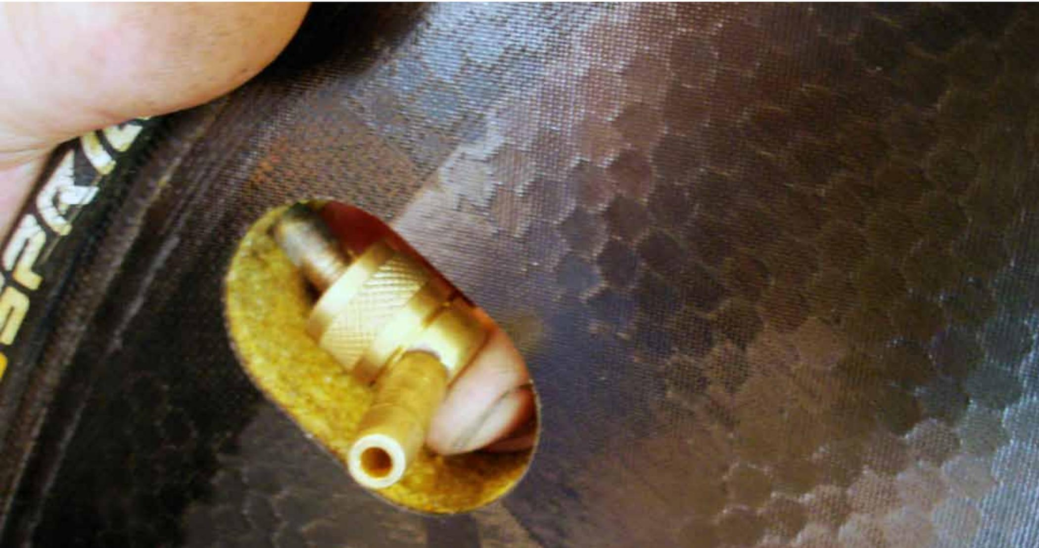
The next step is getting the angle pump adapter onto the valve of the disc.
