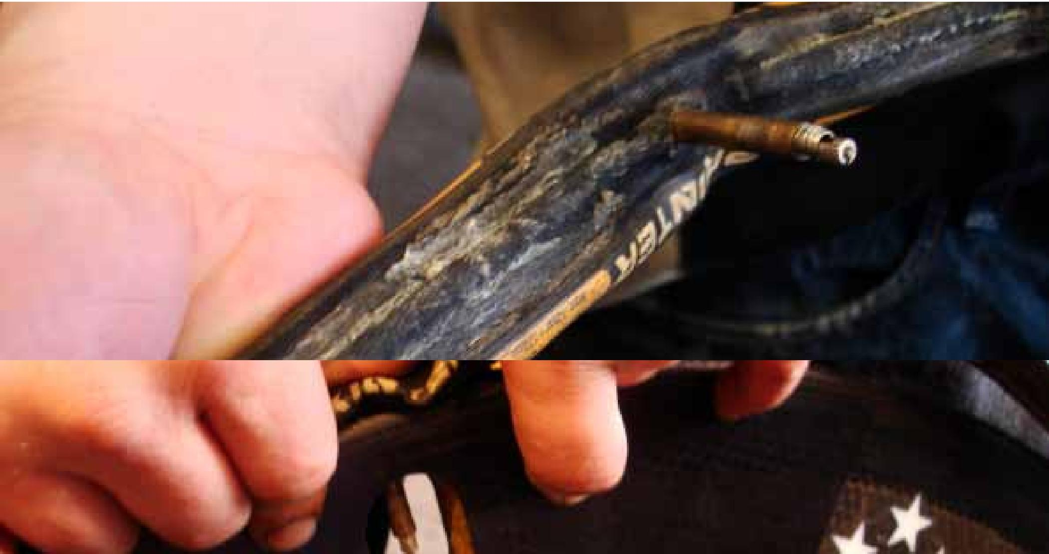
Once getting the flattened tire off, open spare, making sure there is a layer of glue on the tire beforehand. Start with the valve hole, by placing the valve in straight.
