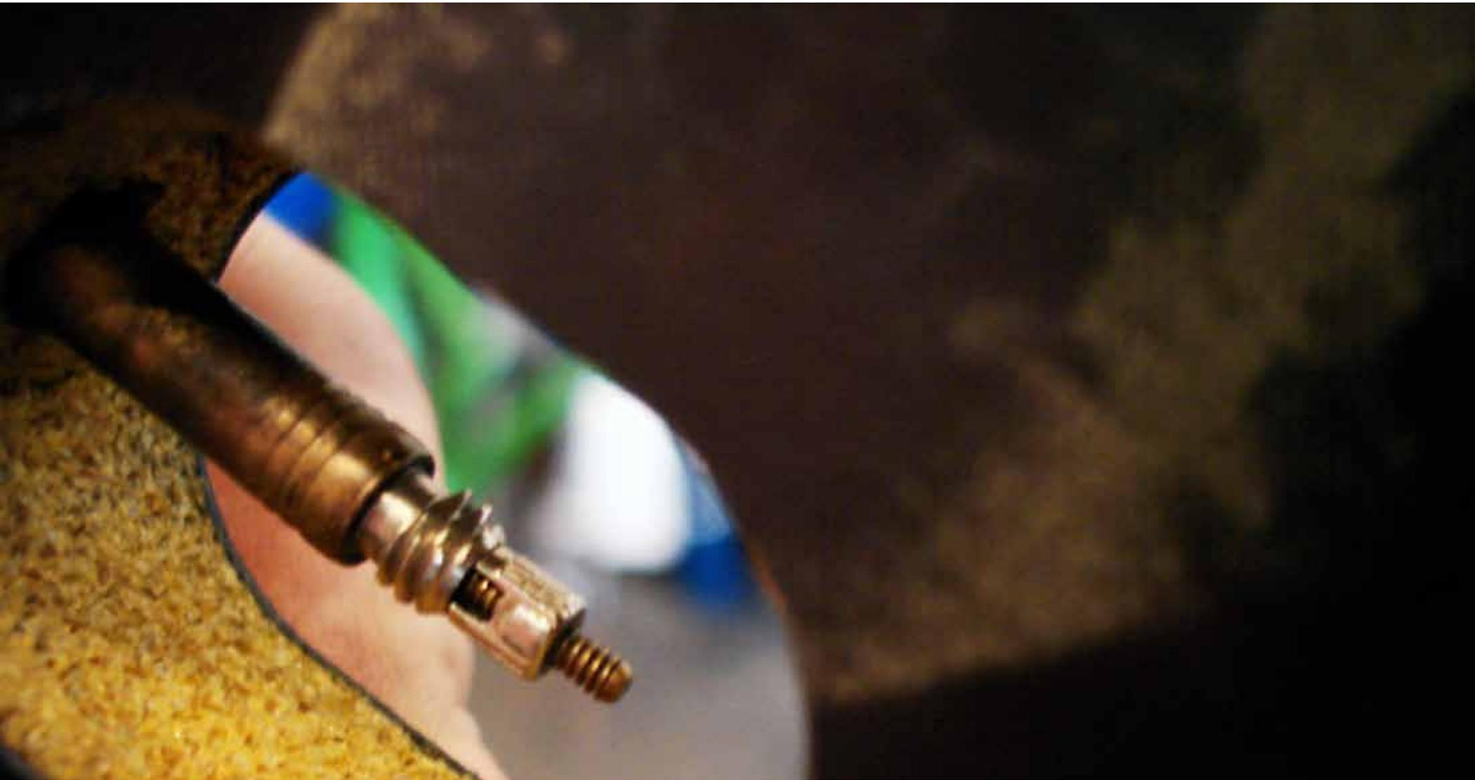
After valve is shut, you can put the wheel back into the bike and be on your way. Its that easy!
