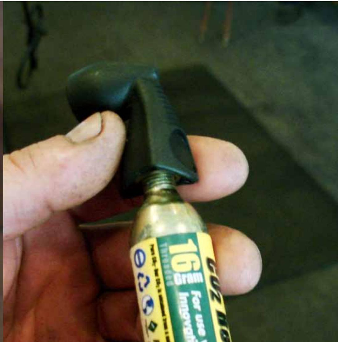
If you have never used a CO<sub>2</sub> inflator before, screw the inflator onto the canister, this will pierce the tank, which stays closed, then to release the air unscrew the cap slightly.
