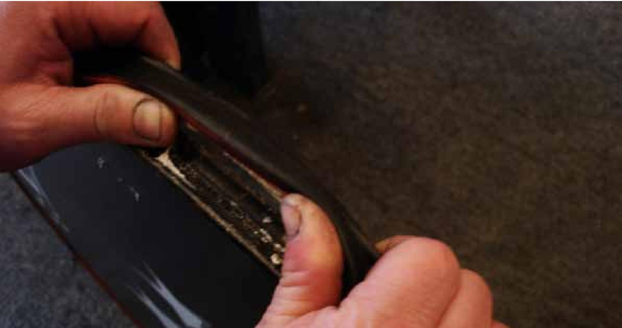
Getting the glue to let go of holding the tire on the rim by bending it back and forth against the direction of the rim and gain more and more leverage.
