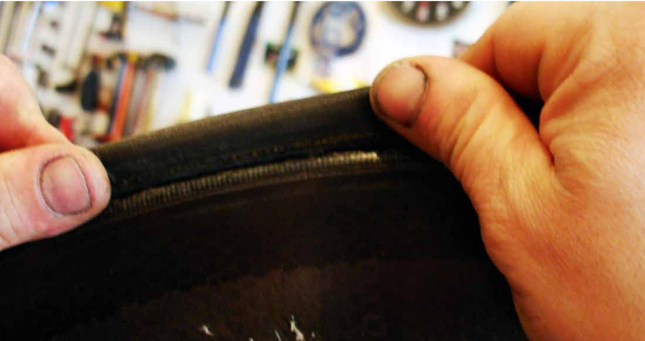
After the tire is on the entire rim, proceed to center the tire on the rim before inflating. The cloth tape on the tire should be showing on both sides of the rim about 3 mm. Check one side and flip the wheel to see if it is even on both sides.
