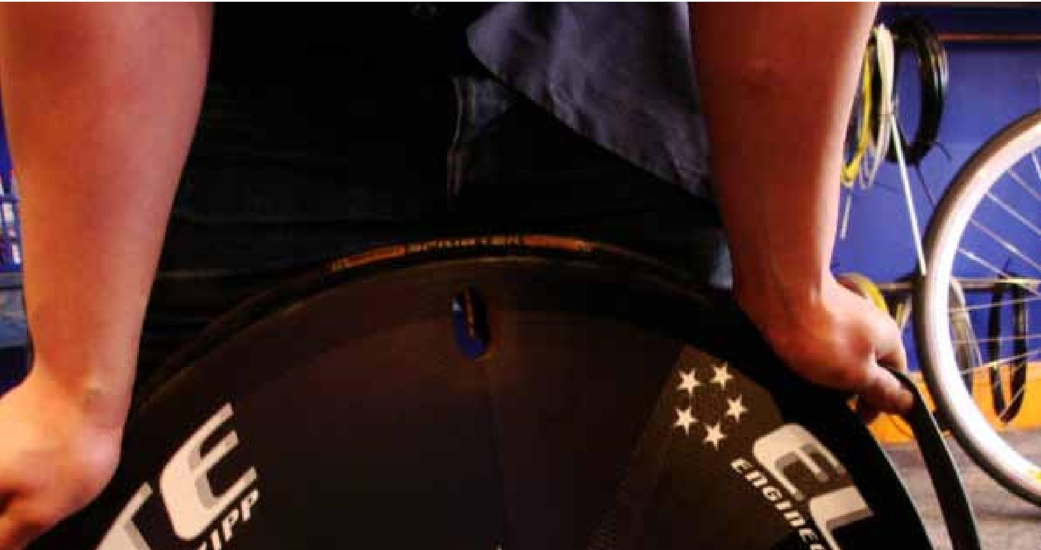
After placing the valve in straight, put equal pressure down heavily on the tire stretching tire over the rim. The more pressure you put in the beginning, the less you will have to use to get the last part of the tire on.
