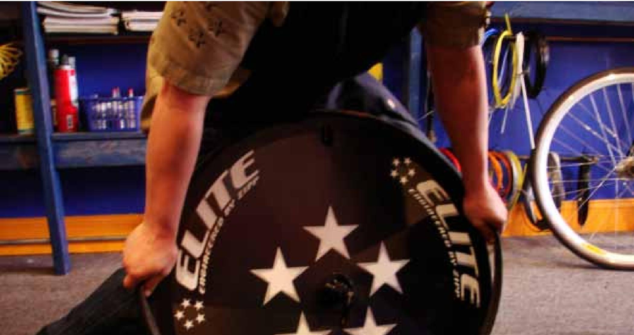
Keeping pressure continually along both sides of the rim it is a good idea to lean the rim against your leg and crouch to get better leverage on keeping pressure on the stretching the tire.
