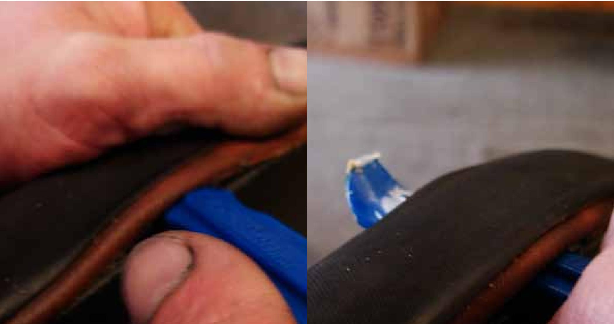
After getting the tire lever under the tire, continue to push back and forth to pull the glue away from both of them, and pull tire to the side using leverage with the tire lever to get the tire coming off the rim to be able to grab it by hand.
