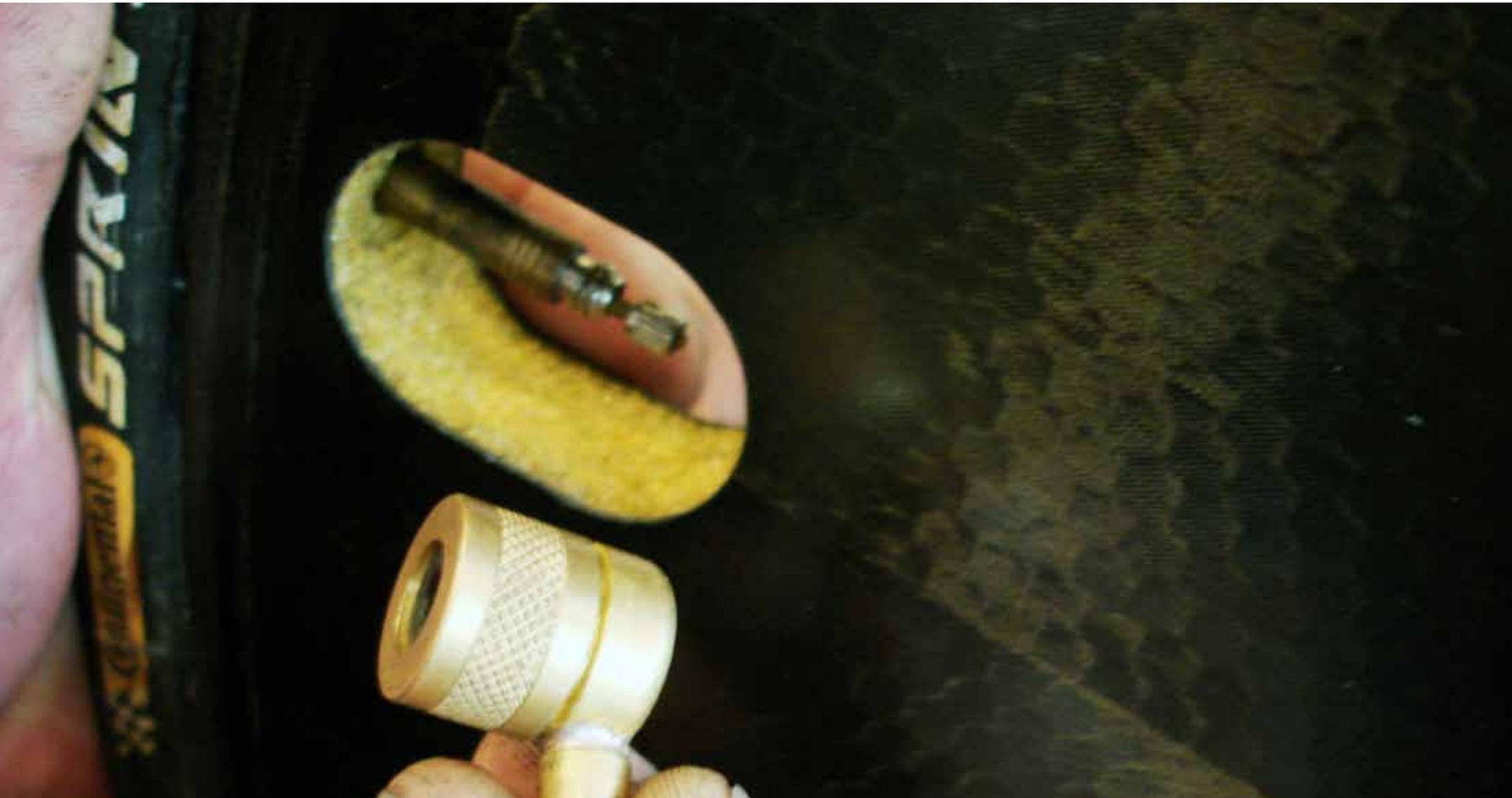
Then you can carefully remove the adaptor and screw the valve down into itself to lock it out.
